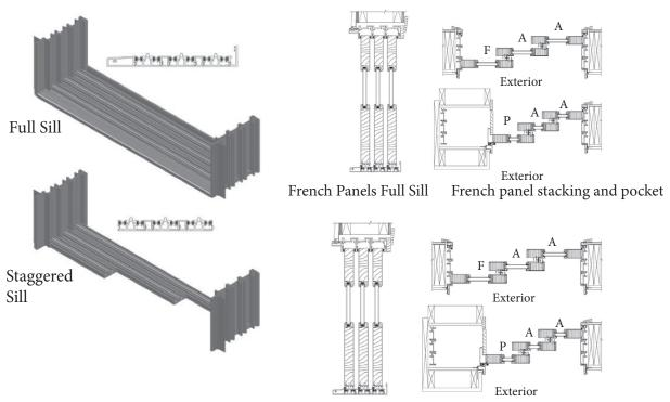
Narrow Panels Full Sill Narrow panel stacking and pocket
